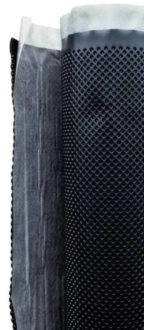
MERZ Drain V consists of a layer of geo-textile fabric in polypropylene and a dimpled membrane of special high-density polyethylene (HDPE). Thanks to special orthogonal discharge channels, it ensures excellent drainage by forming a chamber that always stays empty, thus allowing higher volumes of drained water compared to traditional dimpled membranes.
